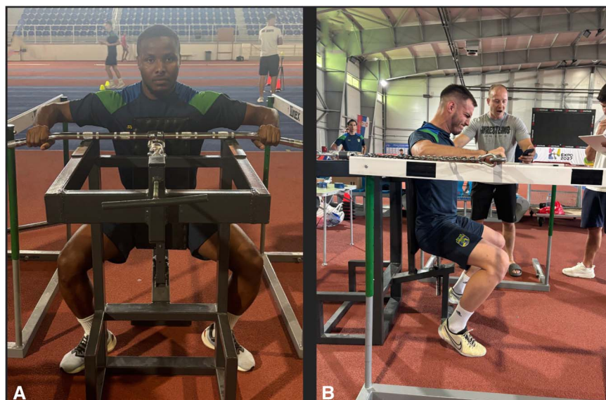
Figure 1. A) Isometric pull test, and B) isometric push test using the DynaMo Max dynamometer attached to the custom-built metal rig.
